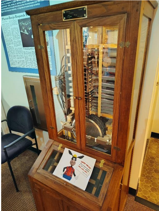
You may have seen player pianos before. This is a player banjo, albeit “out of order” when I was there.
